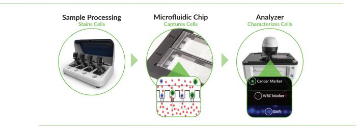
on differences in size and deformability and enable cellular and genomic analysis at the singlecell level. The analyzer imaging station automatically captures bright field or fluorescence images of cells, while its software allows specific analysis and reporting of the results. A recent study by Gogoi, et al. in human patients with cancer confirms the high sensitivity (94%) and specificity (100%) for CTC detection using the Celsee Genesis System.<sup>2</sup>
